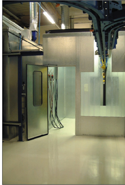
The dry filter two-station manual Eurospray 'Whisperbooth' low-noise spraybooth (left), which utilises Ransburg electrostatic application equipment from ITW Industrial Finishing, and the adjacent paint mixing room, which houses three airless pumps from Wwa.
